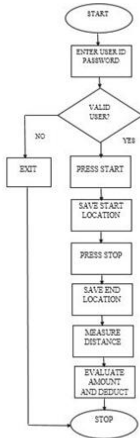
Fig. 6. Dataflow diagram of distance calculation
